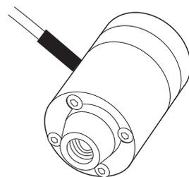
The air sensor 940 used for sample application should be connected on the sample inlet tubing between a selected inlet valve (V1, V2 or V3) and the sample vessel. The air sensor is used to detect when the sample vessel is emptied, and to protect the column from air bubbles. The flow path in this air sensor has i.d. 4 mm.
