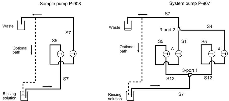
Fig 5-7. Piston rinsing system
