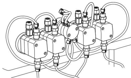
A buffer in an external vessel is drawn in by the action of the pump. Twin reciprocating pump heads then work in unison to deliver a smooth, low-pulsation flow from the pump outlet manifold.
