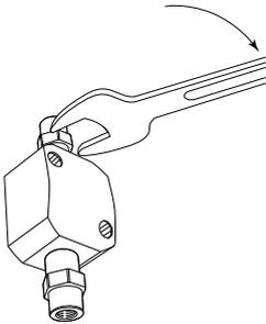
**CAUTION!** Handle the check valves with care when they have been removed from the pump heads to prevent loss of any internal components.
