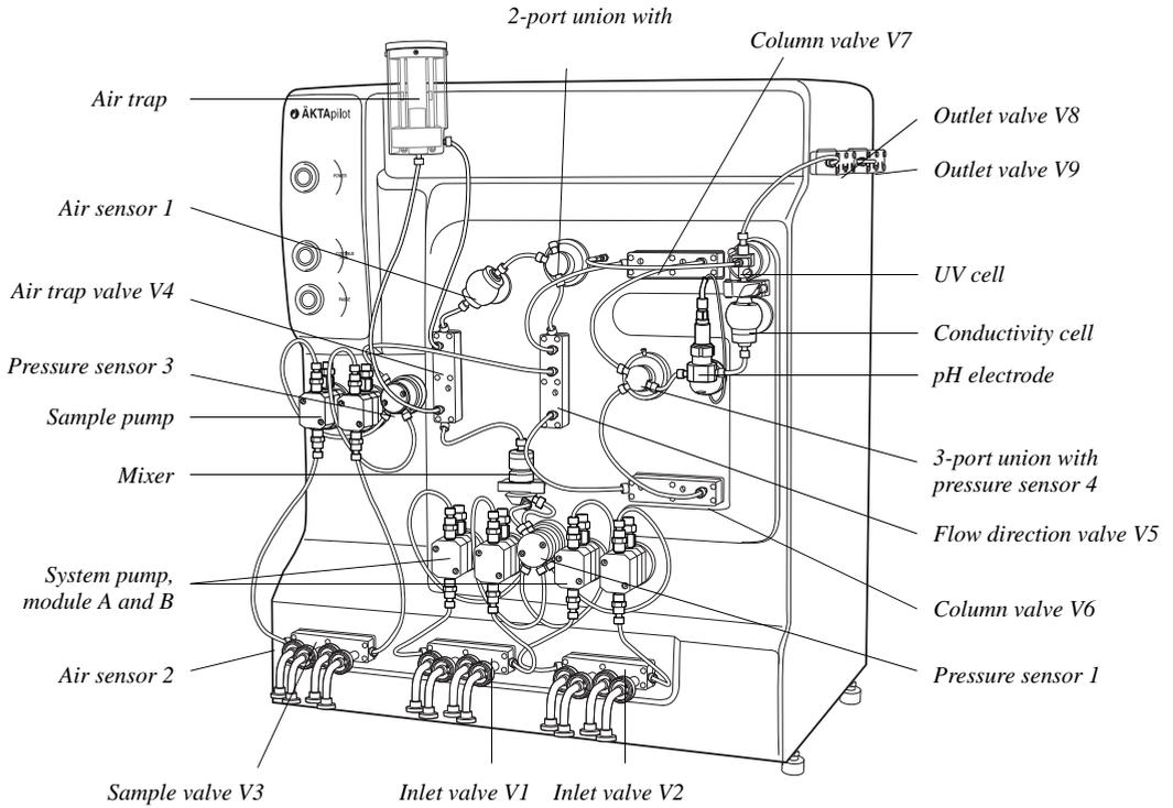
**Fig 5-2.** Location of the ÄKTApilot components
