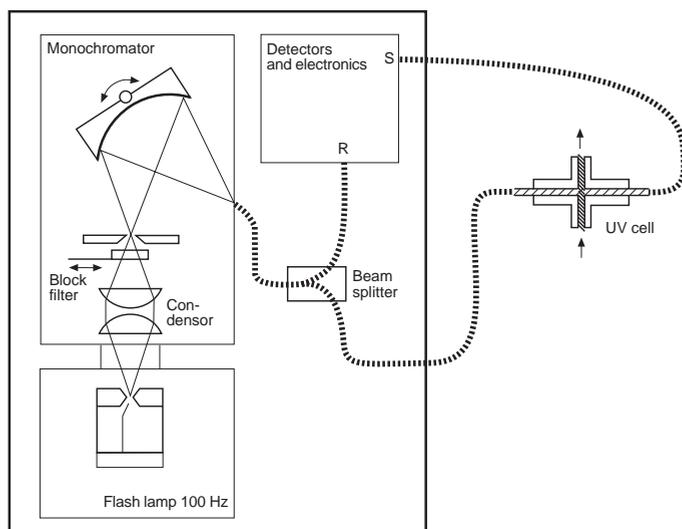
Fig 5-10. UV monitor principle
