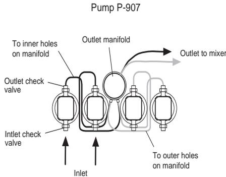
Solvent is drawn up into the pump head through a non-return inlet check valve by the action of the piston being withdrawn from the pump chamber.
