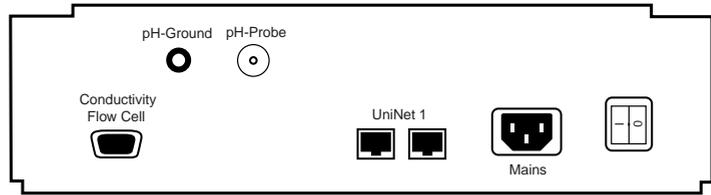
Fig 5-5. Controller mid rear panel
