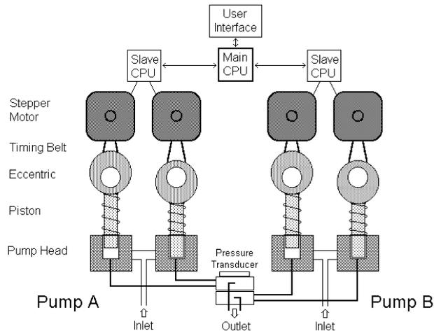
**Fig 5-9.** P-907 pump principle
