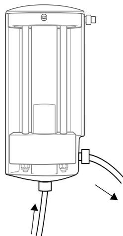
The air trap also has an air vent connector at the top, which is used for adjusting the liquid level in the air trap to suit the flow rate that is used.
