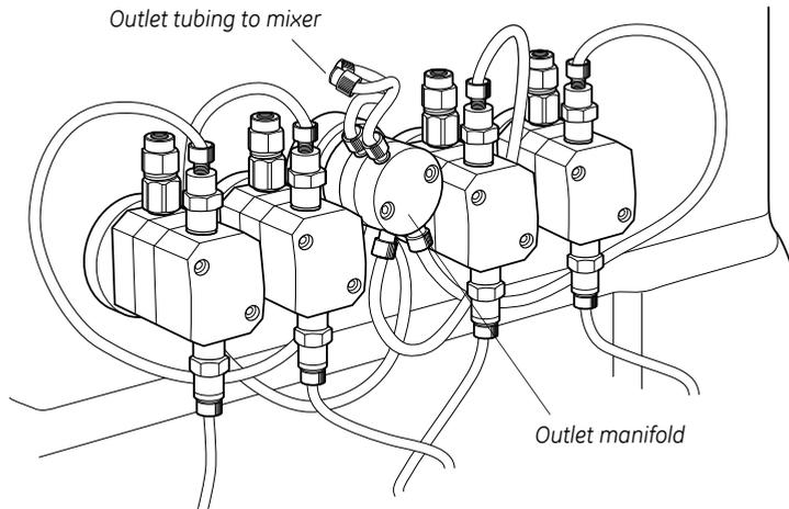
Each outlet manifold also contains a pressure sensor. On P-907, the pressure sensor, which is located in the rearmost part of the outlet manifold, is connected to the left-hand pump module (A).
