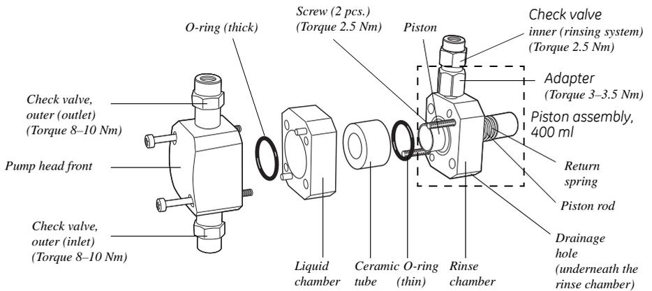
**Fig 3-1.** Pump head, exploded view
