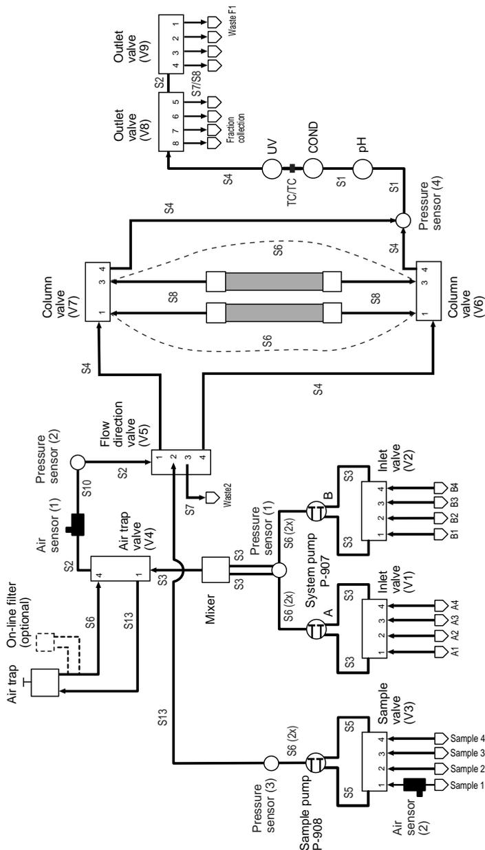
Fig 5-6. Liquid flow path
