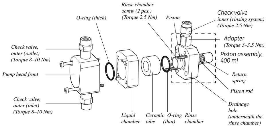
Fig 3-2. Pump head, exploded view
