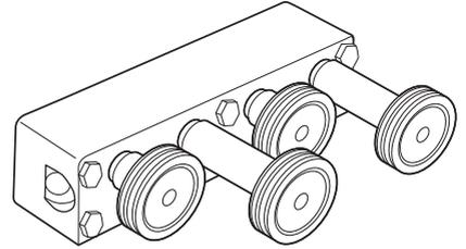
A valve block consists of a connection block containing the ports and the membranes, and a mechanical housing containing the stepper motors, cams and actuating pistons.
