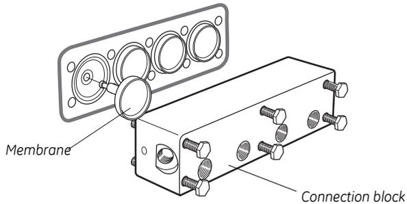
**Fig 3-3.** Valve block, exploded view
