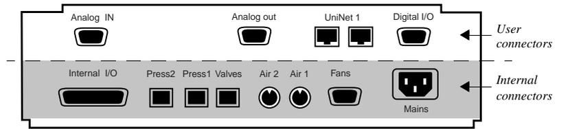
Fig 5-4. Controller upper rear panel
