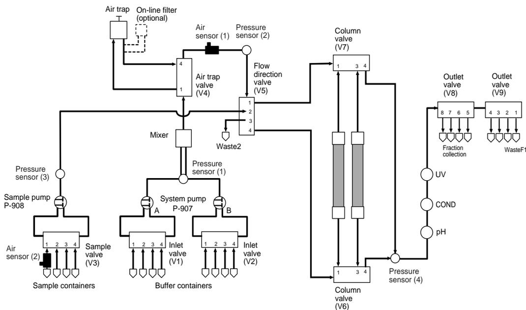
Fig 1-4. The liquid flow path of ÄKTApilot
