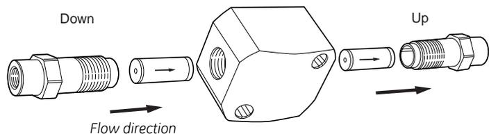
The inlet check valve is fitted to the lower side of the pump head. Tighten the valves using the torque wrench. See Fig. 3-2 for the tightening torque values.
