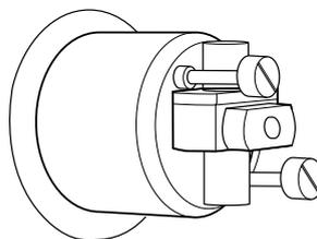
The UV cell housing is made of PEEK, other wetted parts are made of glass and titanium.
