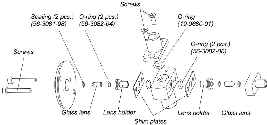
**Fig 3-4.** UV cell, exploded view
