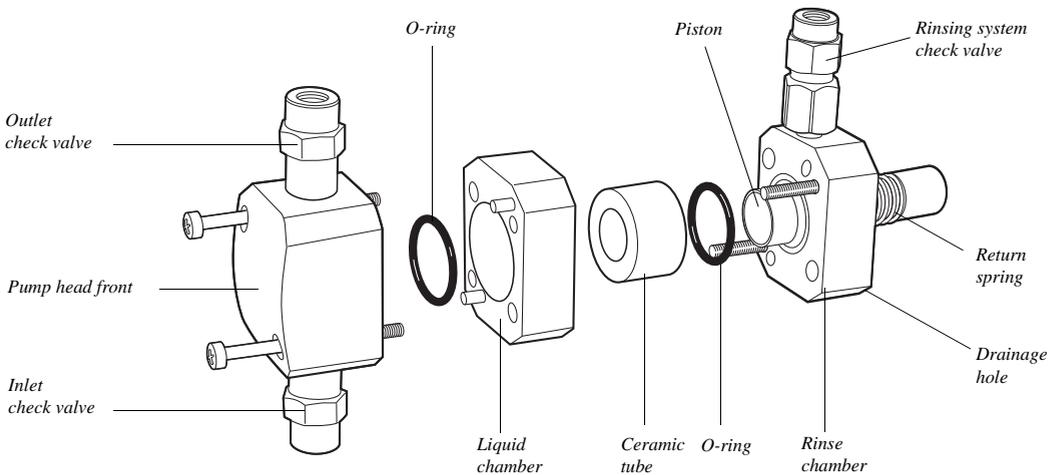
**Fig 5-8.** Pump head, exploded view
