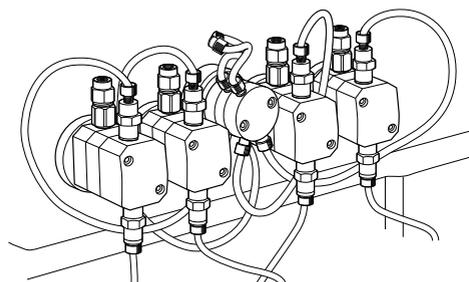
A pressure sensor (Press1) is connected to pump module A (the left-hand pump heads). The pressure sensor can be used in combination with an over-pressure alarm function, which is controlled from UNICORN.
