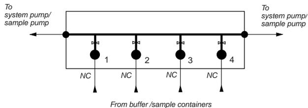
In V1, V2 and V3, only one valve in a block can be open at a time.
