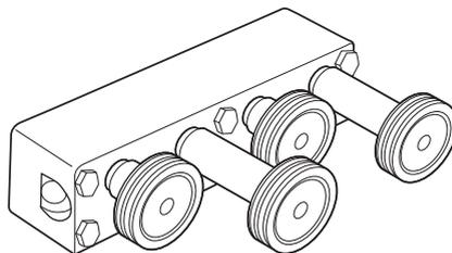
The valve blocks have different numbers of inlet and outlet ports depending on their position in the flow path.
