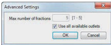
Check **Use all available outlets** to use all the outlet positions installed on the instrument except for Outlet **1-Waste**.
