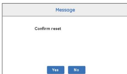
Tap **Yes** to confirm the reset if the valve has been replaced.
